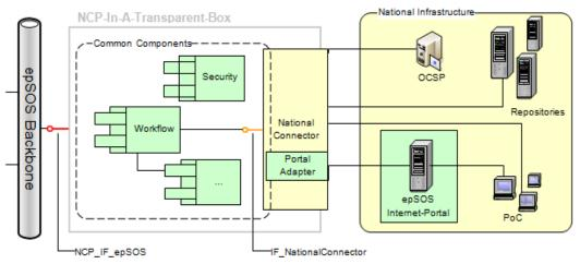
Figure 1: Conceptual Architecture of eHealth DSI NCP Gateway
